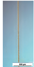
Gorilla® Glass 3 (7 Newton Load)
